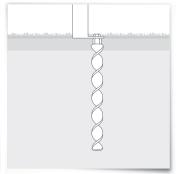
**ground anchors** securely fixes the dugout to grass surfaces.
